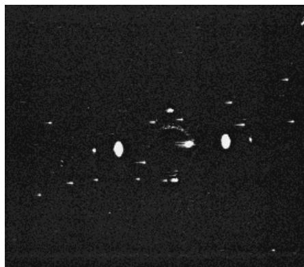
Figure 3 Wide angle X-ray scattering (WAXS) film pattern of uniaxially stretched HNBR-1.
